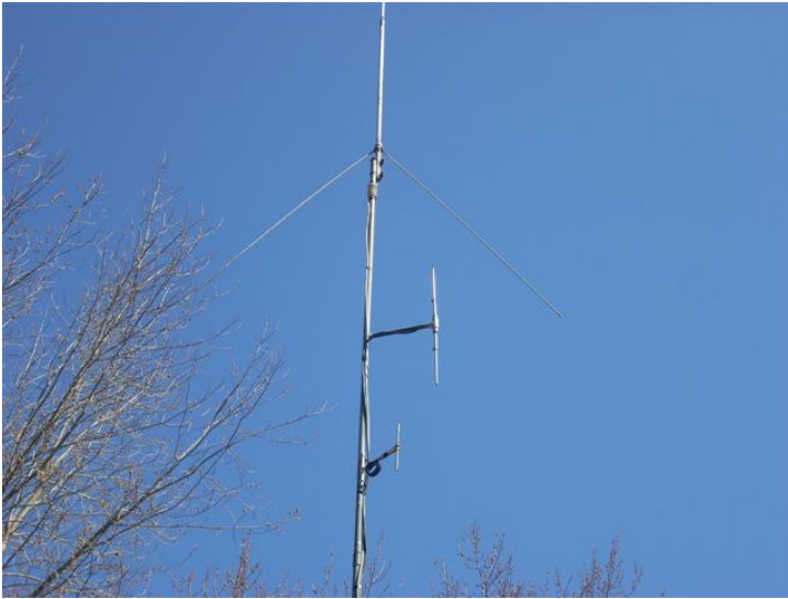
Finished product. 10 meter Vertical on top, followed by the 2 meter dipole and lastly, the 440 Mhz dipole
